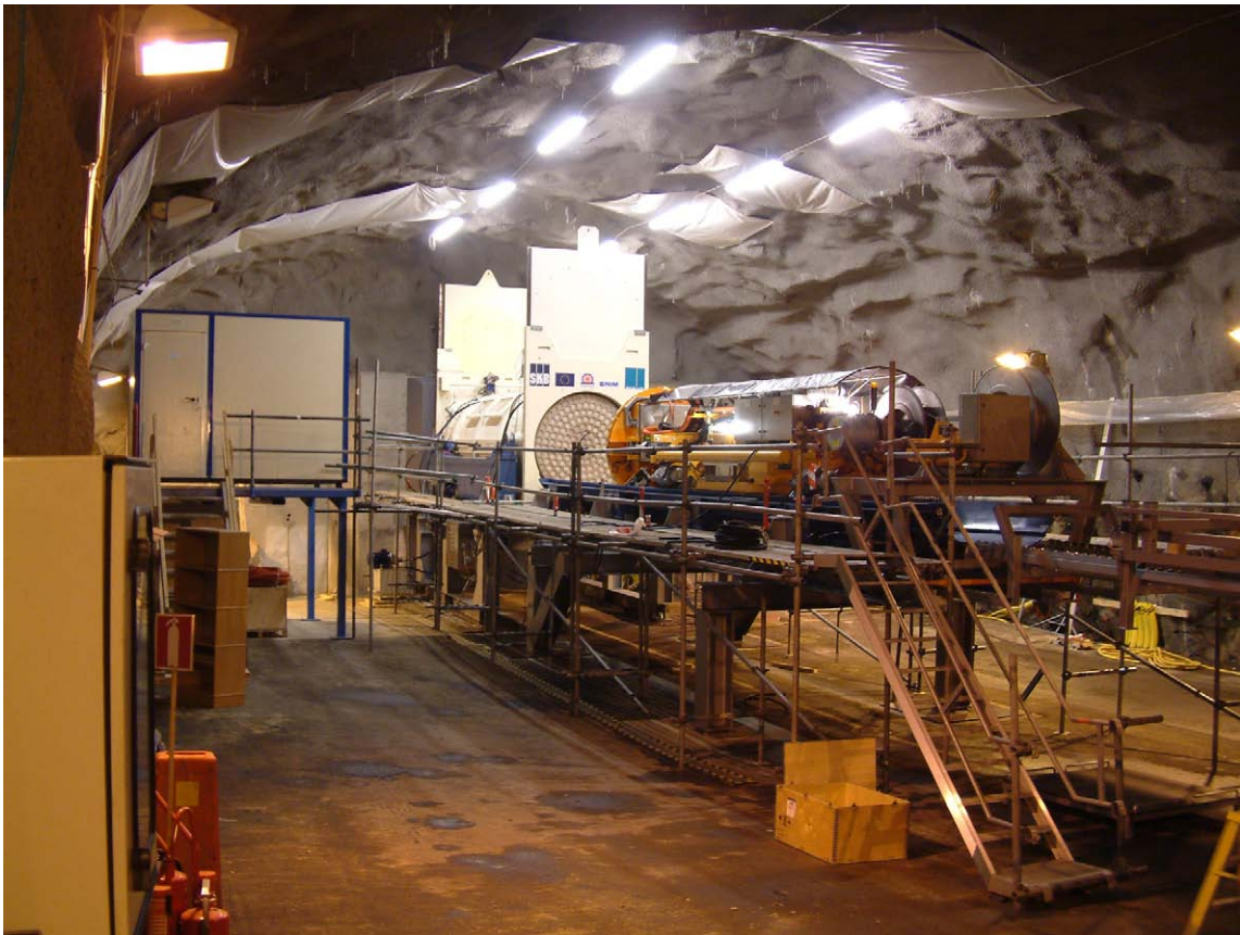
Figure 5-1 Deposition equipment in position (KBS-3H).
