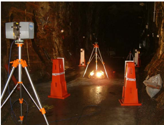
Laser scanner (left) combined with digital camera on a separate tripod (middle) in the TASQ-tunnel
